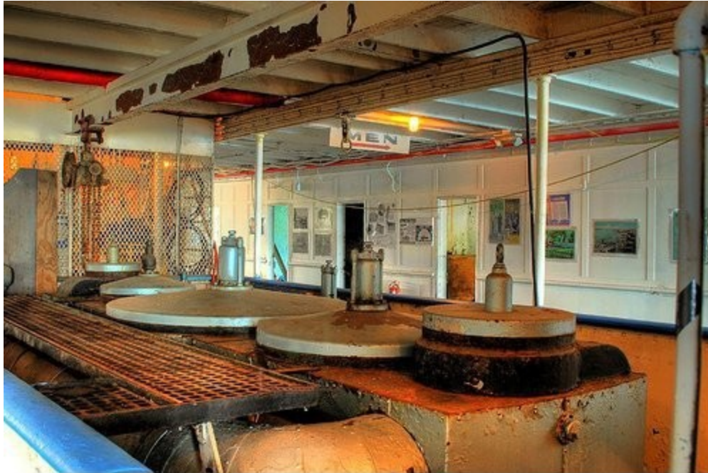
Top of Triple expansion steam engine below. The boats Stopped running:in 1991.
